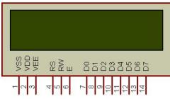
The most commonly used Character based LCDs are based on Hitachi's HD44780 controller or other which are compatible with HD44580. In this tutorial, we will discuss about character based LCDs, their interfacing with various microcontrollers, various interfaces (8-bit/4-bit), programming, special stuff and tricks you can do with these simple looking
