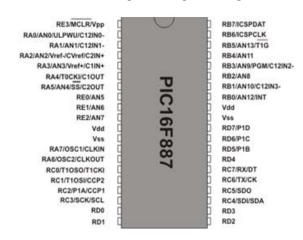
This small trick is often used because it makes the microcontroller package more compact without affecting its functionality. These various pin functions cannot be used simultaneously, but can be changed at any point during operation. The following tables refer to the PDIP 40 microcontroller.
